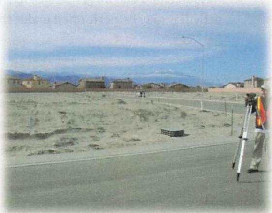
Dynamic Consulting Engineers, Inc. (DCE) uses conventional equipment, total station and GPS to construct topographic maps illustrating the existing characteristics of the site, including topographic contours, natural features, vegetation and trees, buildings, roadways, utilities, and associated elevation and attribute data. These topographic surveys provide the basis for all subsequent project site design and engineering. **DCE also provides aerial survey by drones including aerial imaging.**
