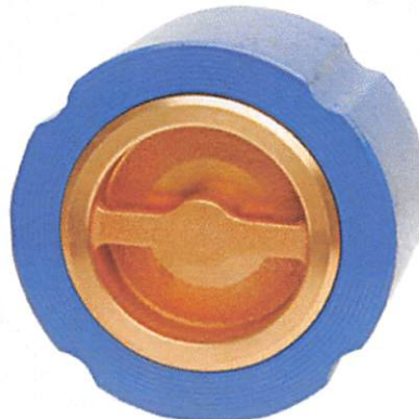
MODEL 888R/888 SIZES 2"- 10" 100% FUSION BONDED EPOXY COATED WITH BRONZE INTERNALS
